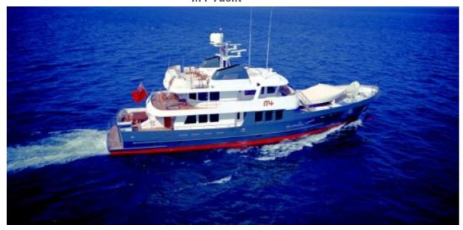
M4 is a 33m motor yacht, custom built in 2002 by RMK Marine. The yacht's interior has been designed by Selldorf Architects and has exterior styling by Seaton Design. M4 yacht has a steel hull with a aluminium / grp superstructure with a beam of 8.53m (27'11"ft) and a 2.87m (9'4"ft) draft .
