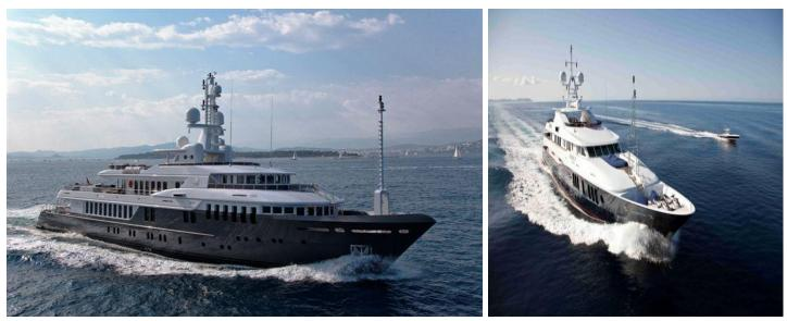
Sea D (formerly Vinidrea II) is a 39.50m motor yacht, custom built in 2002 by Proteksan Turquoise. Sea D yacht has a aluminium hull with a aluminium superstructure with a beam of 8.31m (27'3"ft) and a 1.80m (5'10"ft) draft .
