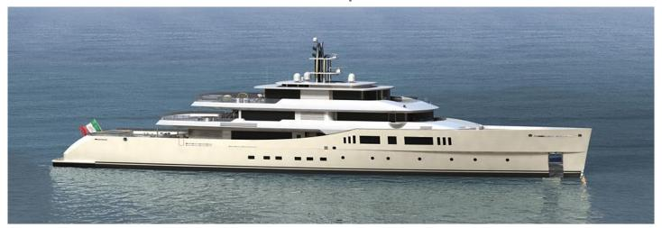
Vitruvius Explorer 73m is a 73m (239'6"ft) motor yacht, due to launch in 2013 from Perini Navi Group. The yacht's interior has been designed by Remi Tessier and has exterior styling by Philippe Briand. Vitruvius Explorer 73m is to have a steel hull with a aluminium superstructure with a beam of 13.3m (43'7"ft).
